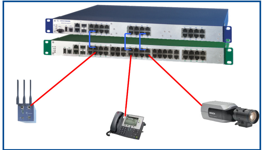
Figure 2.6: PoE midspan power insertion
