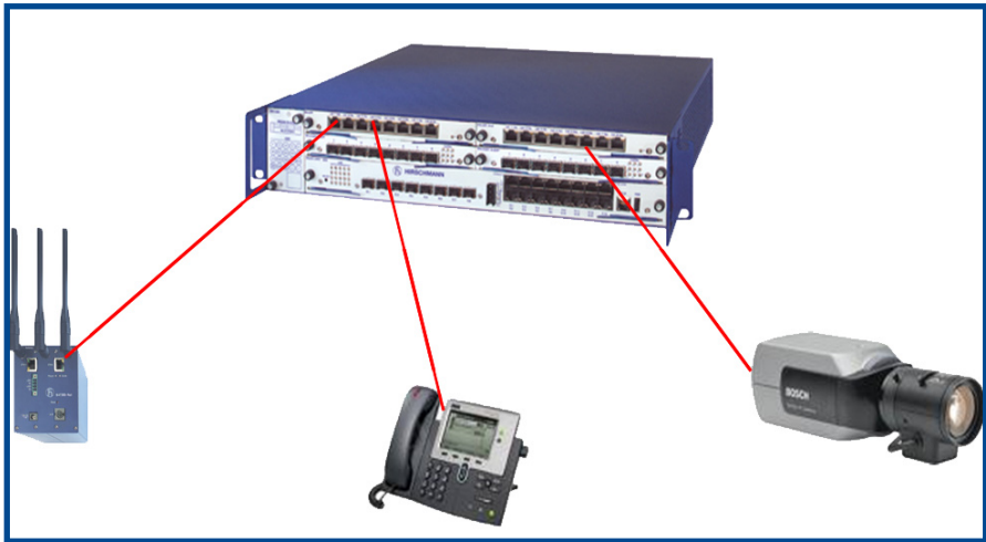
Figure 2.7: PoE endspan power insertion
