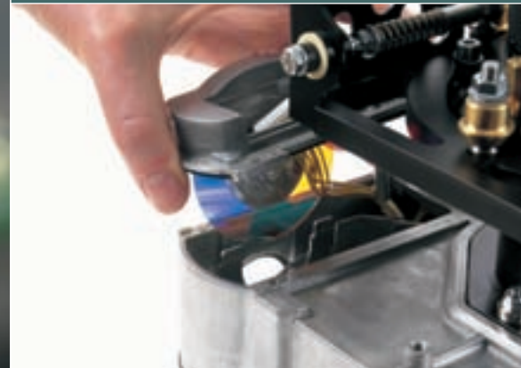
The color wheel can be swapped within seconds.
