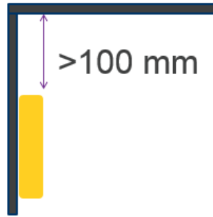
Figure 21: Keep Air Interface away from nearby metals
